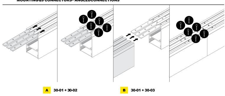
many typesof connections possible, thanksto a variety of angled connectors: 45 deg/ 60 deg/ 90 deg/ 120 deg/ 135 deg/ 180 deg
