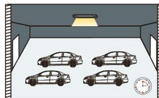
3 After elapse of hold time, the sensor dims the light at a low light level if no new motion is detected.
