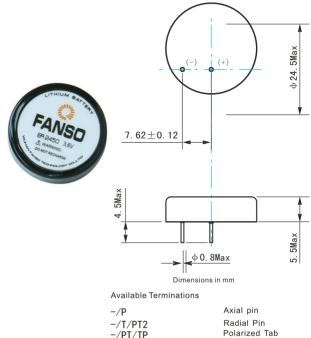
Special terminal can be made according to customer's requirement
